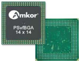
Continued development resulted in Amkor entering the second generation of PoP applications where new memory architectures, required in mobile multimedia applications, demand higher density stacked interfaces in combination with PoP mounted area and height reductions. The previous PSvfBGA and PSfcCSP structures limited the ability of the memory interface to scale in density and pitch, resulting in the need for a new bottom PoP structure.
